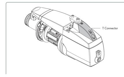
AC VERSION: Plug the T-connector into the serial communication port and carefully check to see that the number on the connector corresponds with the machine-feed number.
