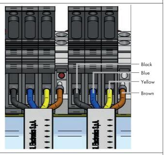
Be sure that flat cables are connected to the transformer with the correct color sequence
