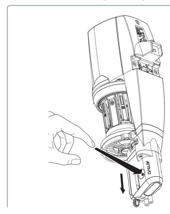
4) Pull the brush to be replaced out of the holder. Insert the new brush by pressing it into its support. Ensure that the ends of the bristles are joined when they are fitted into the ring.
