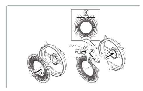
Note: The brush is fitted with a step. The bristle must be fitted with the step facing the drum.
