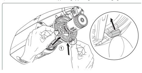
2) Pull the knob with one hand and simultaneously remove the bristle brush.
