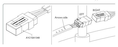
The CAN is terminated with a resistor on the cable, so DS4 must be OFF on all feeders. If one or more DS4 are ON, this will produce a decrease of the BUS resistance, thus leading to communication problems.
