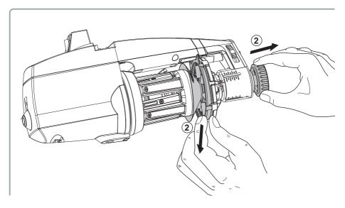
3) If the ATTIVO brake is provided, press the release button. The lights will begin to flash fast. The TWM brake opens. It is only possible to act on the TWM unit when the flashing changes from fast to slow
