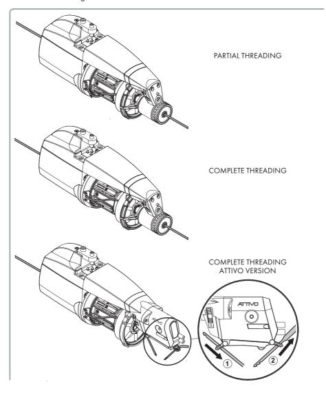
To avoid damaging the TWM we recommend use of threaders that are in good condition with no yarn accumulation around the threader-ends. Use of iron needles for threading must absolutely be avoided as they are liable to damage the TWM.
