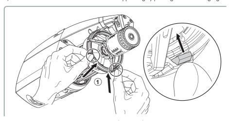
2) Pull the knob with one hand and at the same time remove the TWM tension modulator.
