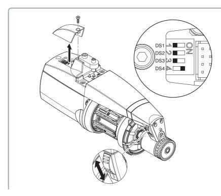
Note: To enable the function performed by each Dip-Switch, the feeder needs to be switched off by acting on switch 0-1; then set the Dip-Switch to the desired position and switch the feeder on again.
