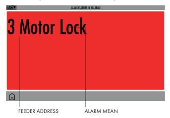
In case feeders are OK, nothing will be shown on the display. Here below a list of the possible alarms:
